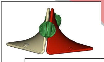
Here are several images of the HyPar Cell. This is one of the most basic building blocks of larger HyPar structures and is a great way to see how HyPars connect and how to use the lettering to make sure you are attaching the Hypars in the proper way.
